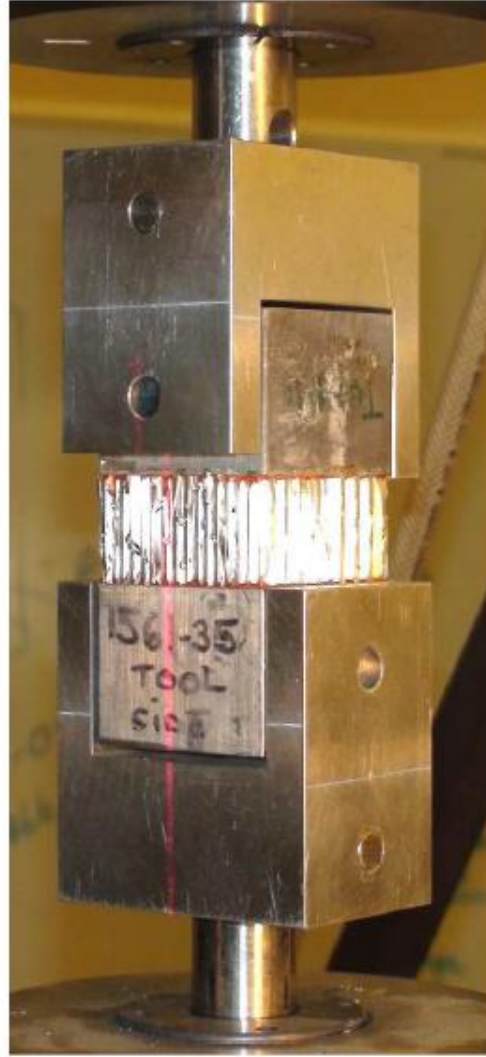
Figure F.1. Flat-wise compression test set-up for the core property determination.
